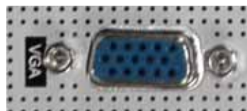
Figure 1.1 Connect to a VGA monitor.
